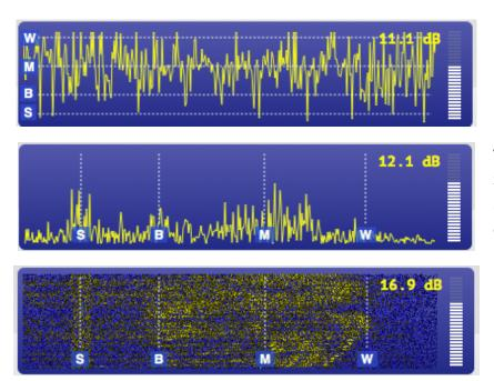
On the left of filter selectors there is a view that displays the signal. It has three modes Scope, Spectrum and Waterfall.
